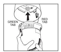
**CAUTION:** Make sure the dome drive locks into place. Pull down on the dome drive with moderate pressure to ensure that it stays in place.
